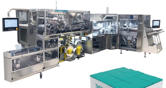
Turnkey system for high-speed primary packaging and cartoning of bouillon tablets
